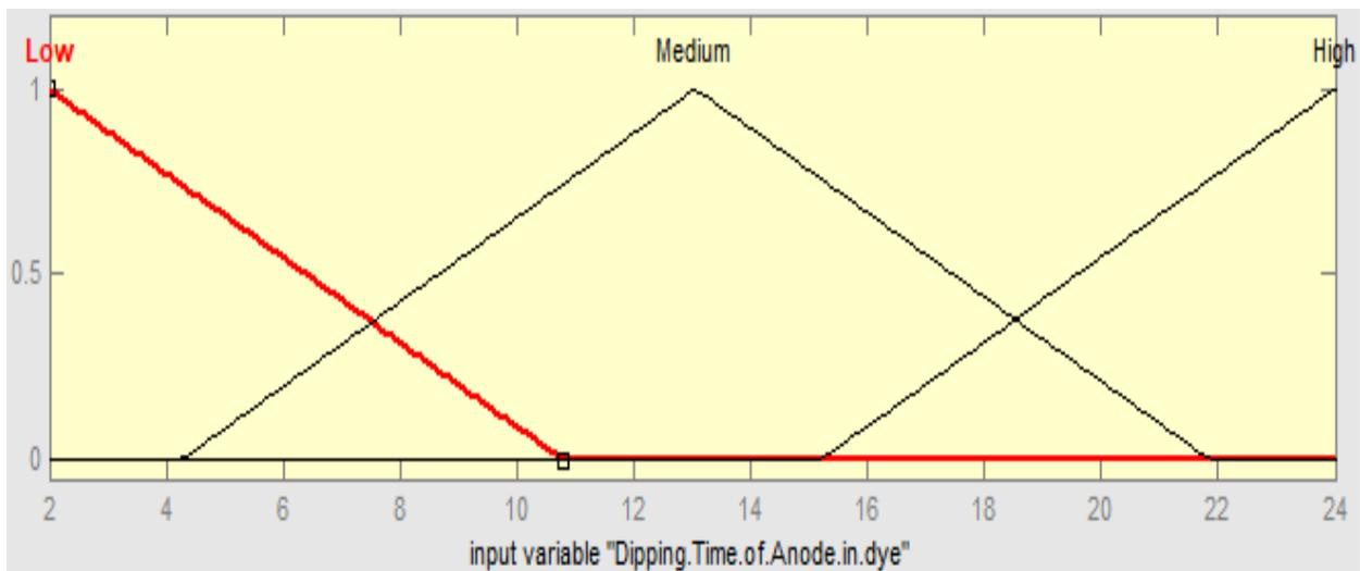
Fig.4: Membership function of input Dipping time of anode in dye
