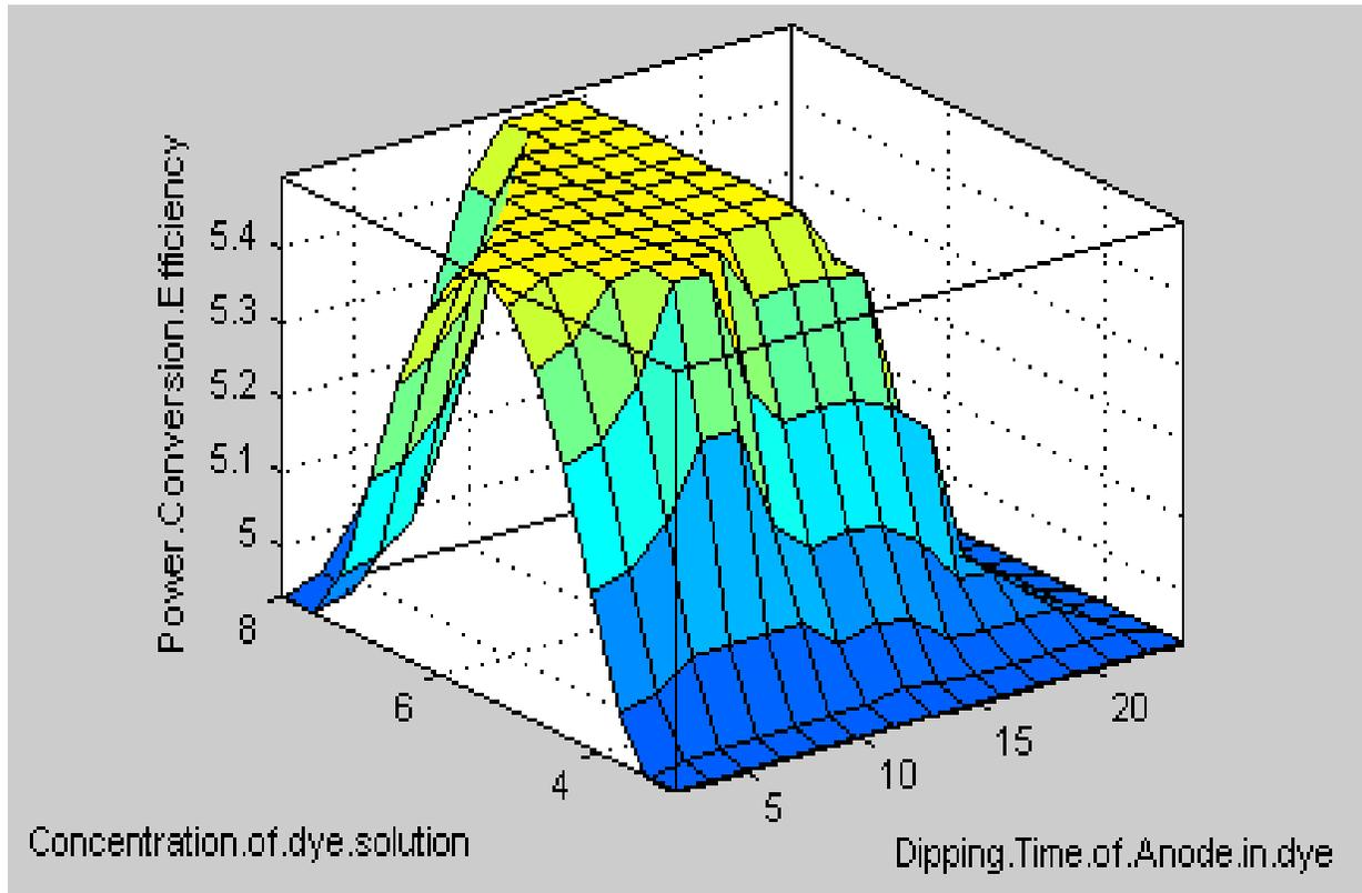
Fig. 8: 3D graph between the input concentration of dye solution and dipping time of the photo-anode with respect to the output power conversion efficiency.
