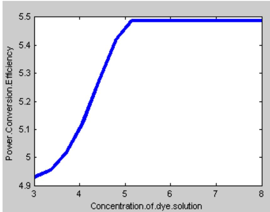
Fig. 6: 2D graphs of output power conversion efficiency with respect to (a)Concentration of dye solution
