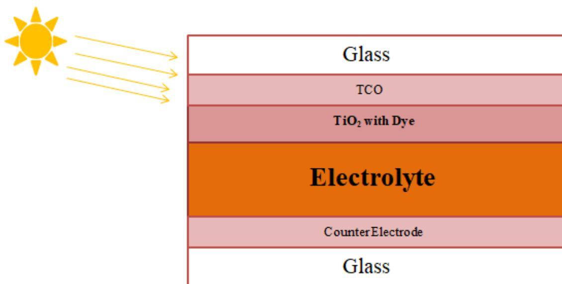
Fig. 1: Components of a typical dye sensitized solar cell
