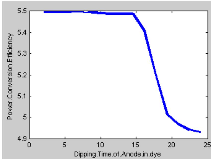
Fig. 7: 2D graphs of output power conversion efficiency with respect to Dipping time of anode in dye
