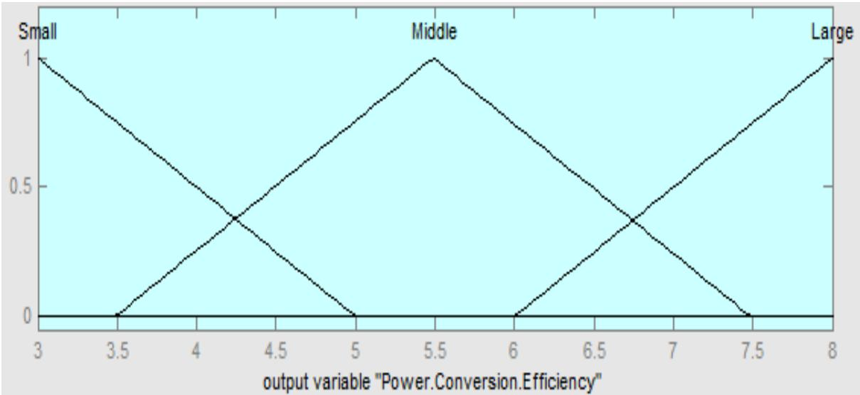
Fig. 5: Membership function for output power conversion efficiency
