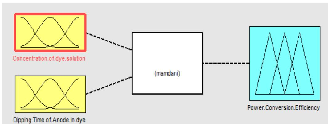
Fig. 2: FIS diagram for the parametric estimation of dye.
