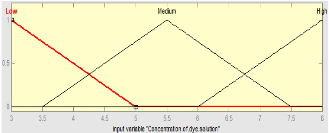
Fig. 3: Membership function of input Concentration of dye solution
