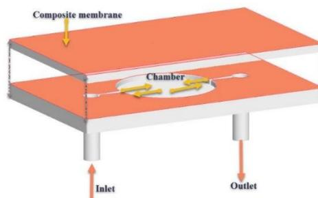
Fig. 2: Schematic diagram of Valve-less Micropump
