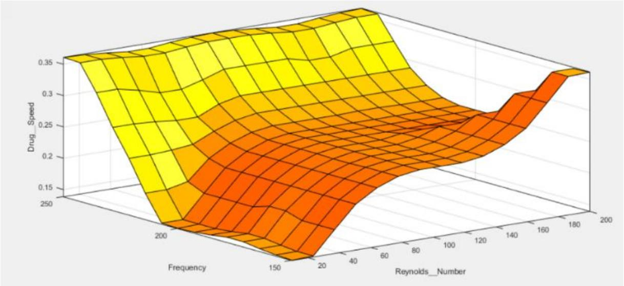
Fig. 11: 3D graph between Reynolds Number and Frequency with drug Speed as output
